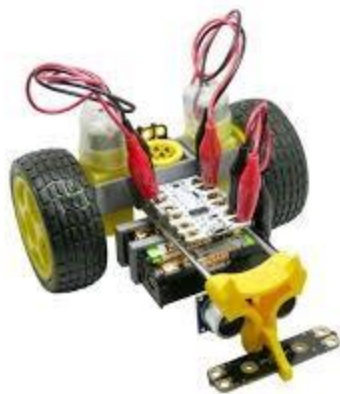
Crumble controllers attached to wheel units – Go Kart kit.
